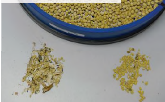
Determination of percentage screenings and foreign matter in sunflower with a 1,8mm slotted sieve.
